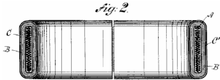
Fig.2 is a horizontal central cross-section of Fig.1
