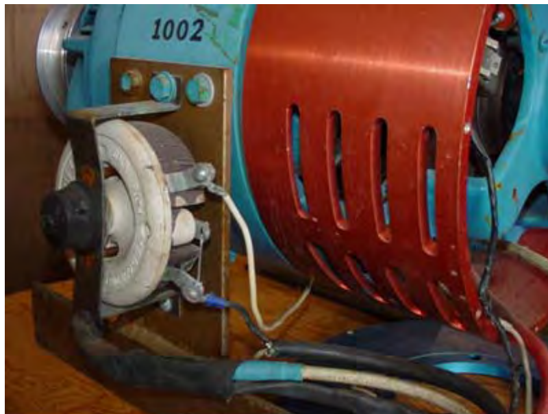
Side Mounted 200 Watt 2 Ohm Rheostat and Attached Cabling
